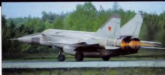
There are many MiG-25s configured for reconnaissance, in a multitude of variants. This MiG-25RBK has a large side-looking radar in the nose.
